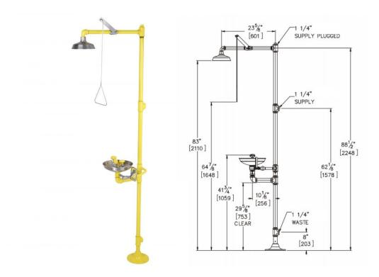
Model S2340 is our combined safety shower and eye wash with stainless steel head and bowl. Complete with stainless steel shower head and bowl and yellow plastic spray heads. Supplied with a 1" chrome plated brass stay open ball valve with stainless steel pull handle and activation lever for the shower and a 1/2" chrome plated stay open ball valve and stainless steel push handle for the eye wash.
